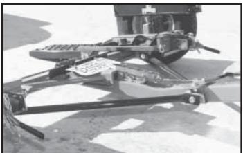
**Step 5.** Grasp bed release handle on tongue and pull toward coupler. This releases the tilt bed to permit loading.
